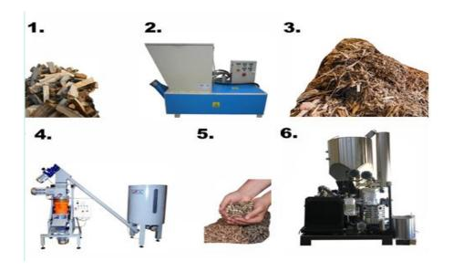
1. Biomass is fed into shredder. 2. Shredder produces biomass stock. 3. The biomass stock that is fed into pelletizer to produce pellets. 5. The pellets are fed into hopper container. 6. The gasifier produces syngas from pellets.
